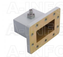
229WCASM Right Angle Rectangular Waveguide to Coaxial Adapter 3.3-4.9GHz WR229 to SMA Male
